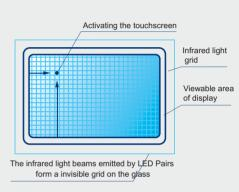
The technology uses infrared emitter-collector pairs to project an invisible grid of light on the screen. When a beam is interrupted, the absence of the signal at the collector is detected and converted to an X/Y touch coordinate.
